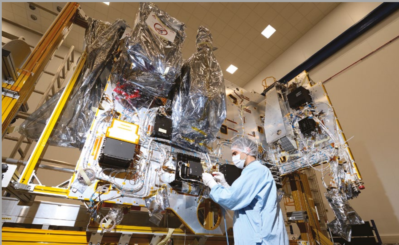
Solar Orbiter instrument panel showing PHI, METIS and SPICE optical units, and a number of instrument electronics units including those for EUI and MAG (Airbus D&S)
