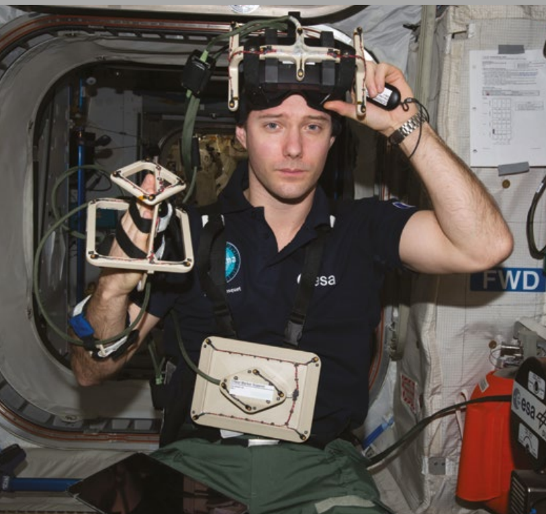
Thomas Pesquet operating the Grasp experiment with a VR headset to test how the brain interprets visual cues without gravity (NASA/ESA)
