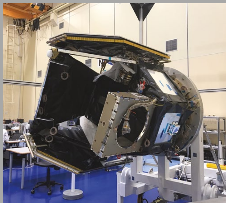
CHEOPS flight platform at Spain during the insulation fit-check (Airbus D&S)
