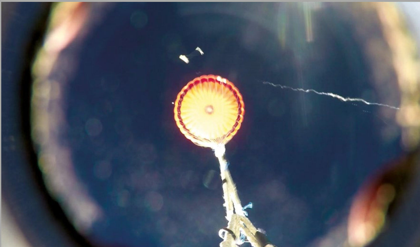
This 1.25-m diameter 'Supersonic Parachute Experiment Ride on Maxus', or Supermax, flew piggyback on ESA's Maxus-9 sounding rocket on 7 April
